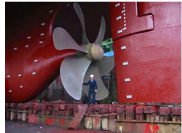
Galvanic anodes placed on a ships hull
