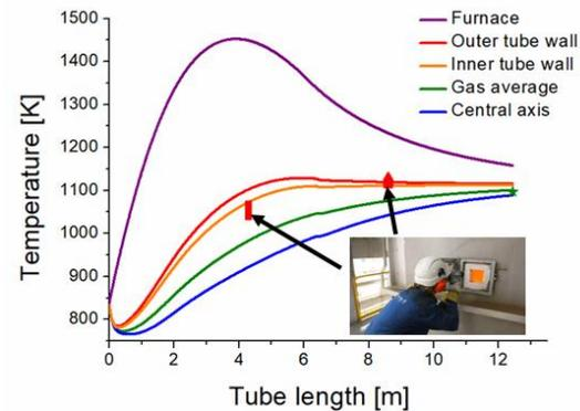
Figure 3. Temperature distribution along the furnace and the catalytic tube. Lines: simulation. Symbols: experimental data.
