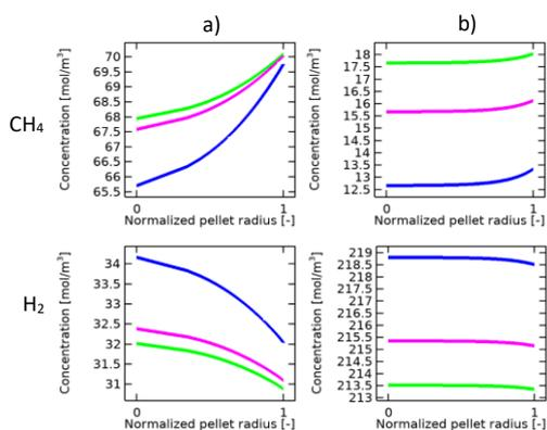
Figure 5. Simulated concentration profiles of  $CH_4$  and  $H_2$  in catalyst pellets at different positions along the tube: a)  $z=0.6$  m (minimum temperature); b)  $z=12.43$  m (outlet). Radial position: tube axis (green line), middle of radius (magenta line), and inner tube wall (blue line).
