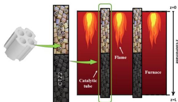
Figure 1. Scheme of a typical SMR reactor. Left: Catalytic pellet. Middle: Detail of a catalytic tube. Right: Scheme of the furnace with the catalytic tubes.
