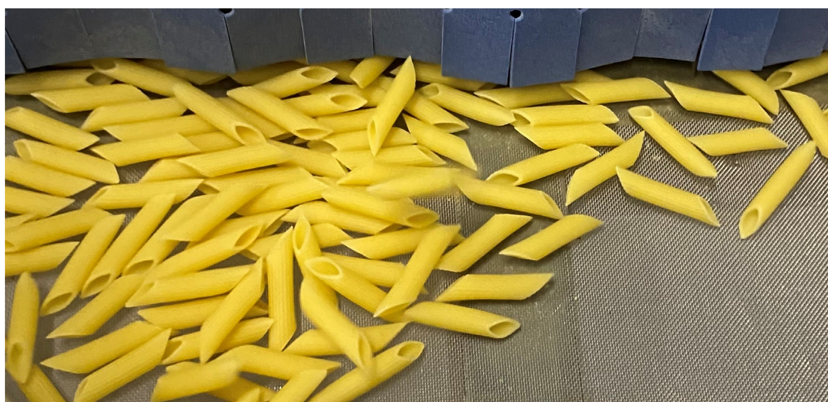
FIGURE 1. Short pasta descends onto a conveyor system designed to transport the product through a drying process that involves the use of hot and moist air.
