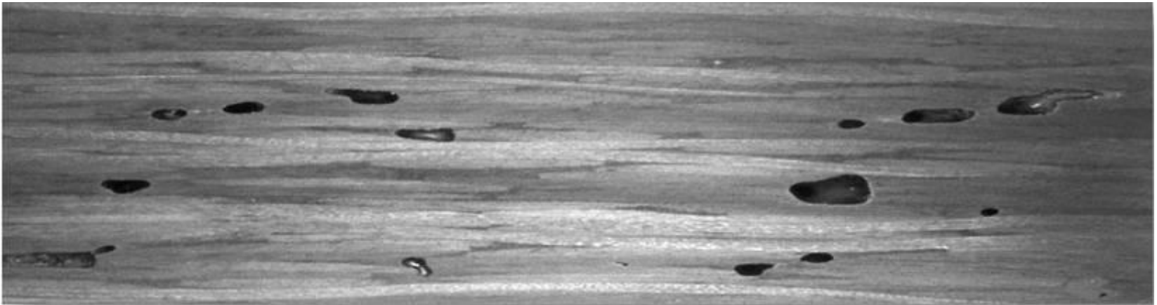
Example of cured Out-of-Autoclave (OOA) prepreg composite with high void content*
