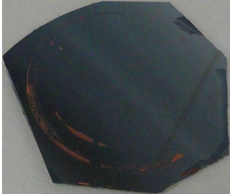
Figure 10. Copper electrodeposited onto Si-substrate
