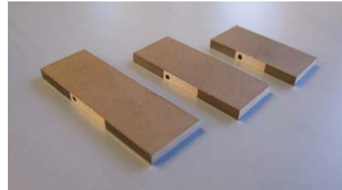
Figure 6 Prototypes of the piezoelectric interleaved multilayer thickness mode transformer of different sizes: 30 mm, 25mm and 20 mm.
