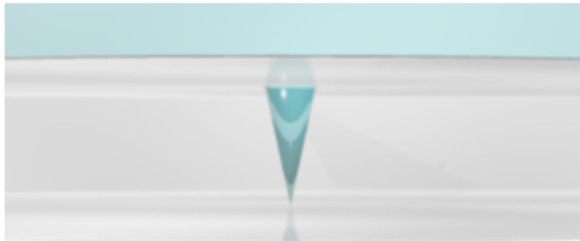
Glass Nanopore Membrane (GNM) Orifice radius: 200-500 nm
