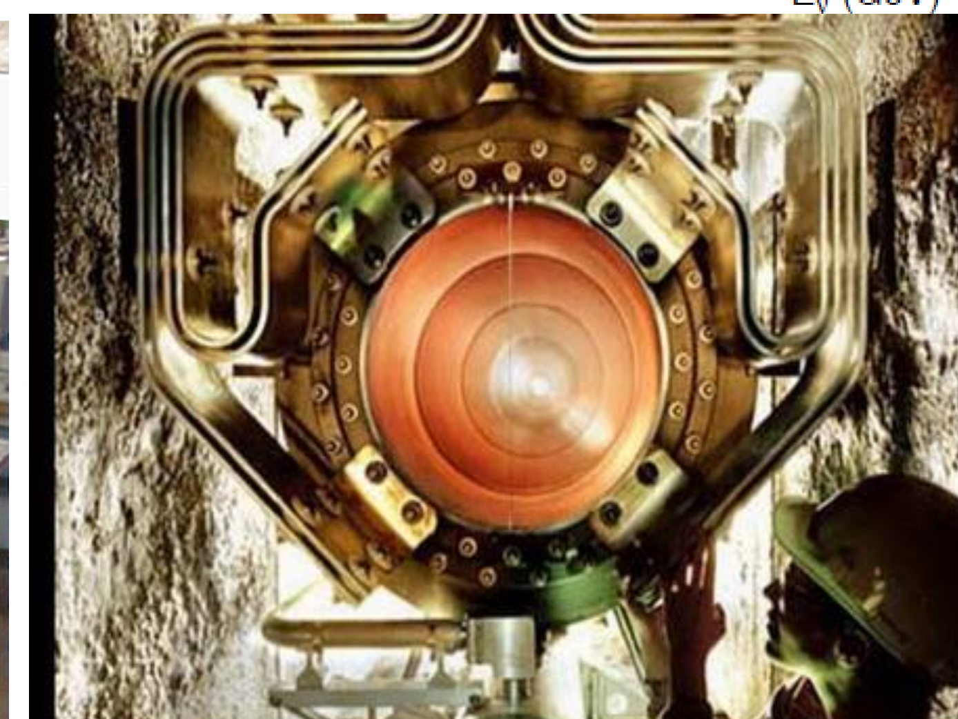
Internal Horn conductor and the full device instrumentation (FNAL)
