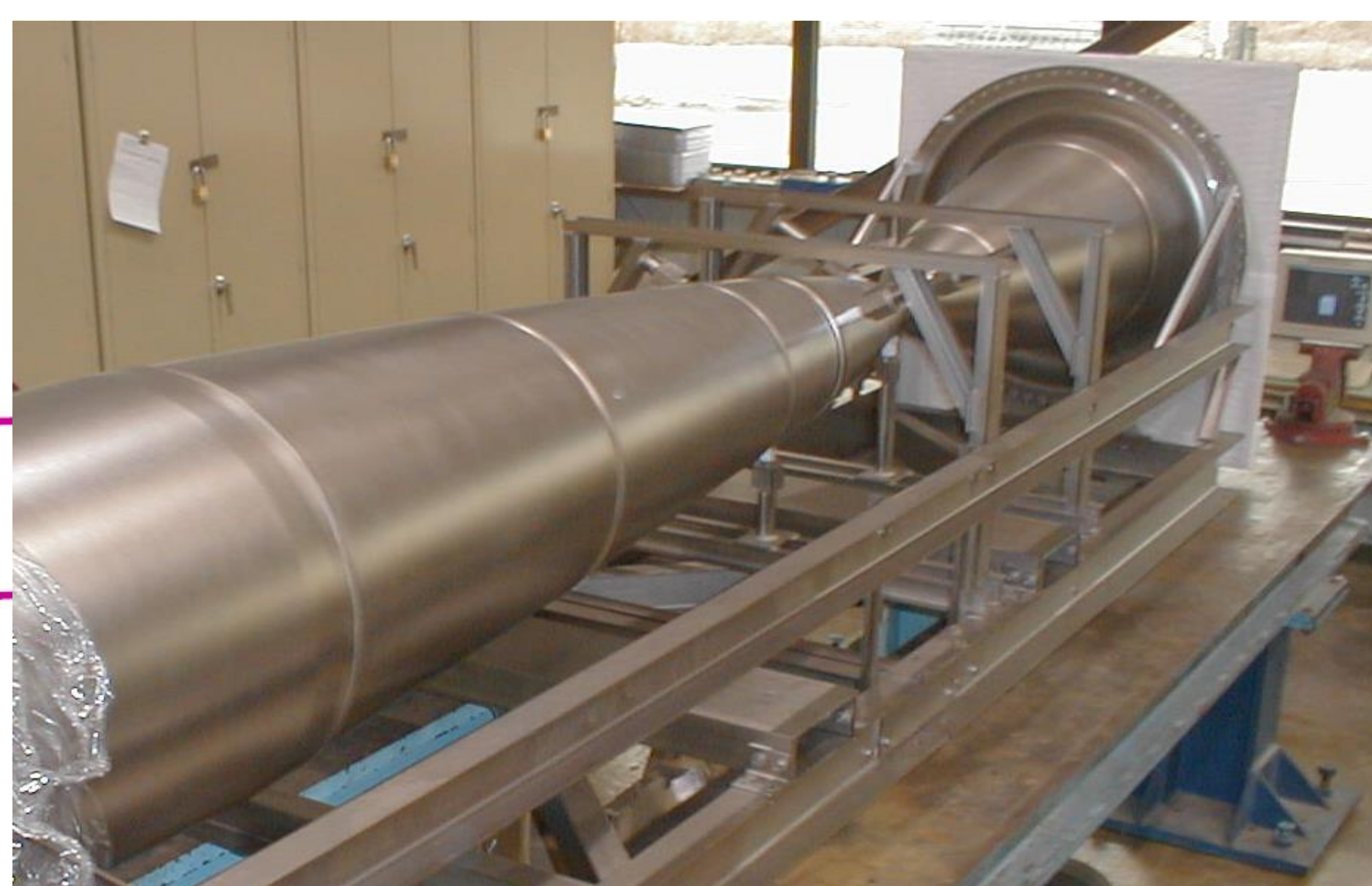
Internal Horn conductor and the full device instrumentation (FNAL)
