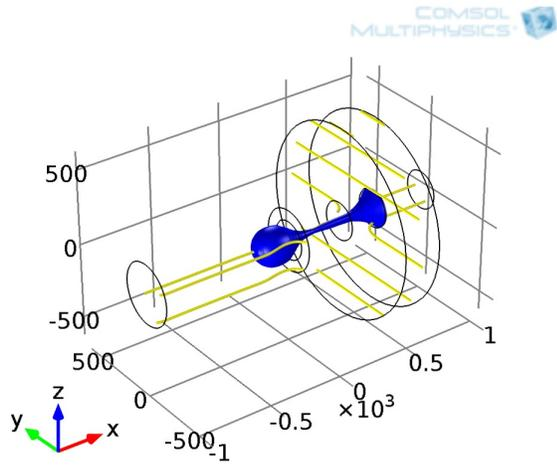
**Figure 2:** Capillary based flow focusing device (Time step 2)
