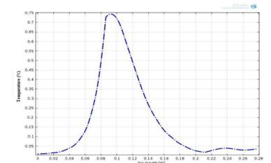
Figure 10. Temperature increase of Omni directional antenna
