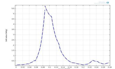
Figure 8. SAR variation of Omni directional Antenna
