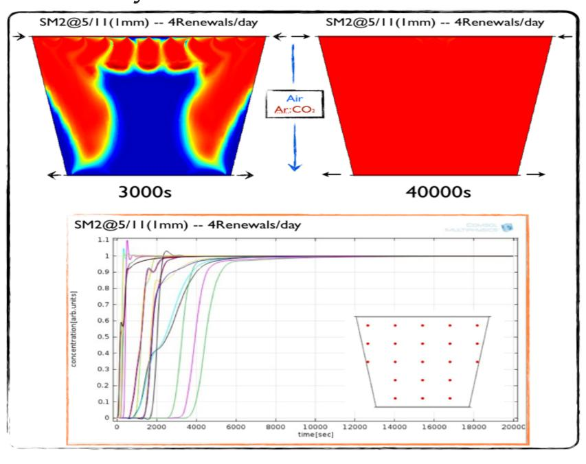
The lower plot shows the normalized concentration of the gas mixture in various points inside the chamber versus time.
