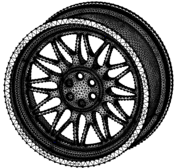
Figure 2 CAD geometry with FEA mesh of typical Automobile Aluminum Alloy Wheel
