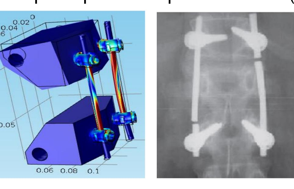
Figure 2. Modeling of a test standard for a spine fixation device, which should be able to predict the possible clinical failure modes.
