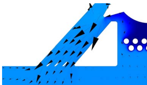
Figure 15. Thermal field and velocity vectors close to the chilled beam (summer).
