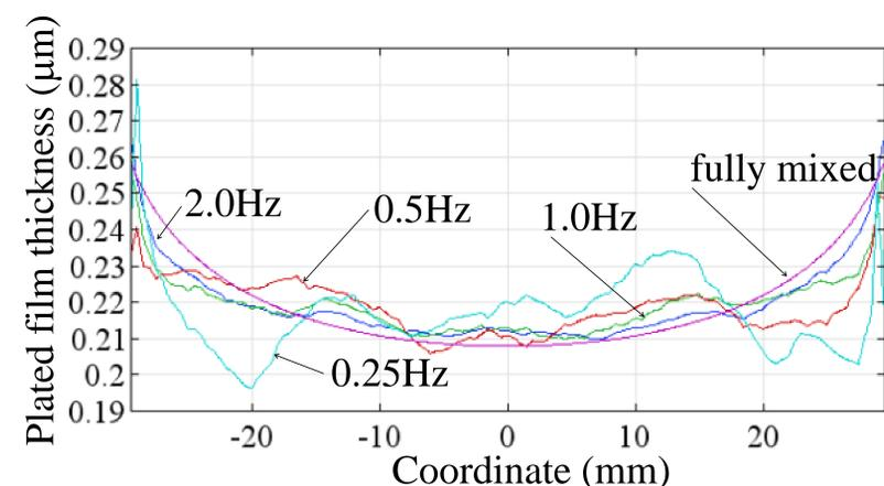
Figure 5. Plated film thickness at the cathode
