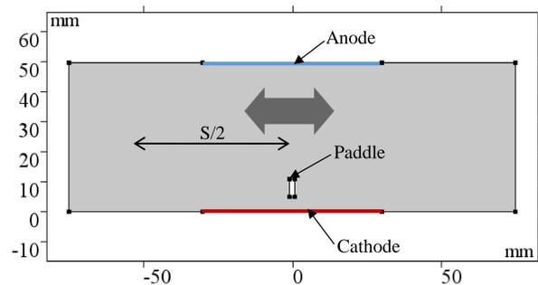
Figure 1. Schematic of a reciprocating paddle electroplating cell.
