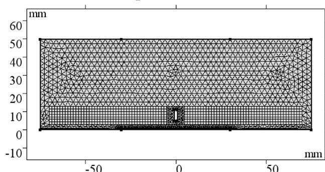
Figure 2. Computational mesh of an assembly geometry based on a reciprocating paddle of original condition
