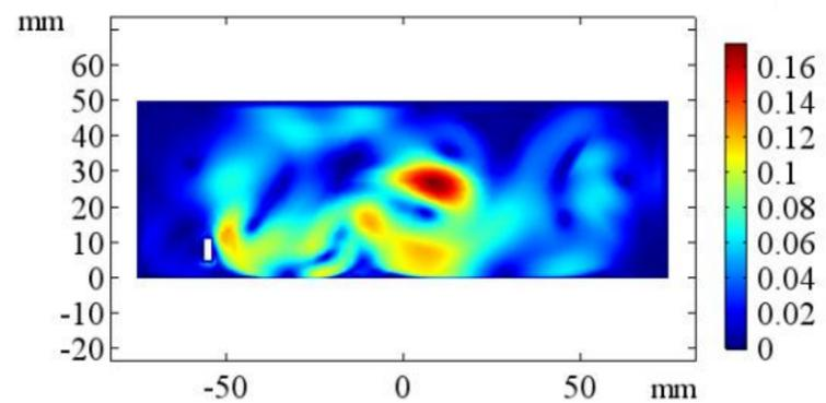
Figure 3. Velocity at  $t = 3T/4$  (T is cycle period).
