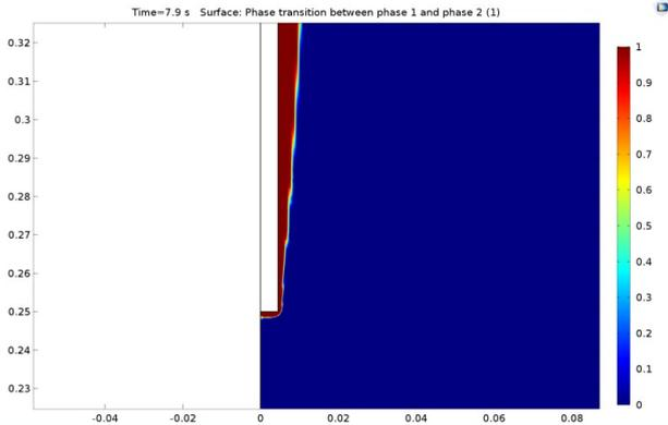
Figure 1: Vapor Film Formation around the Heated Cylindrical Rod
