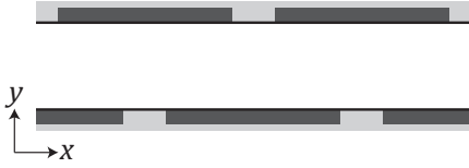
Figure 1: One periodic segment of the zig-zag traveling wave pump. Light gray and dark gray represent the substrate layers (glass or plexiglass) and the electrodes (gold), respectively. Black lines correspond to solid-electrolyte interfaces.
