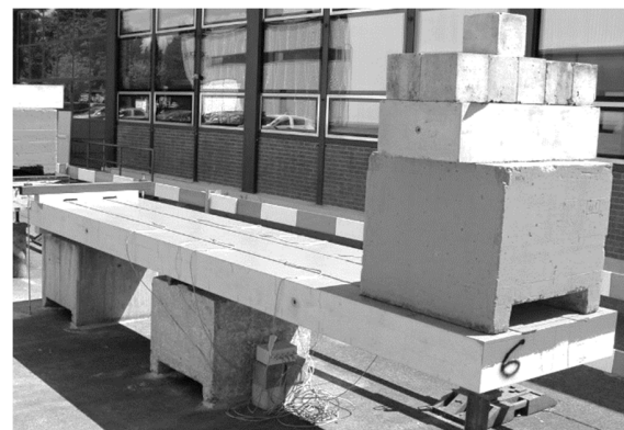
Figure 2. Long-term experimental set-up, simulating a CFRP strengthened lateral cantilever.
