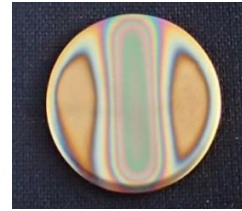
Figure 5: Specimen coated in the demonstrator with plates at 385°C, 500 Pa and with gas flows of 450 sccm (main nozzle) and 450 sccm (ring nozzles)
