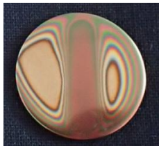
Figure 4: Specimen coated in the demonstrator without plates at 385°C, 500 Pa and with gas flows of 450 sccm (main nozzle) and 450 sccm (ring nozzles)
