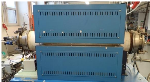
Figure 3: CVD reactor at the gemeinnuetzige KIMW Forschungs-GmbH
