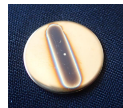
Figure 6: Specimen coated in the demonstrator with plates at 385°C, 500 Pa and with gas flows of 125 sccm (main nozzle) and 125 sccm (ring nozzles)
