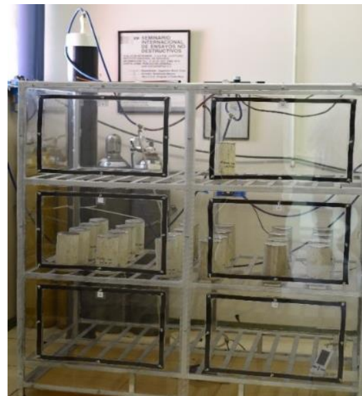
Figure 2. Accelerated carbonation chamber used in the experimental work.
