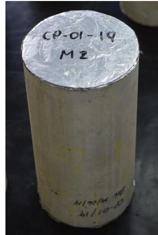
Figure 1. A cylindrical sample of concrete with its bases recovered by aluminum foils.
