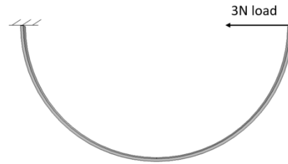
Figure 3. The geometry and boundary conditions of the rotary spring model
