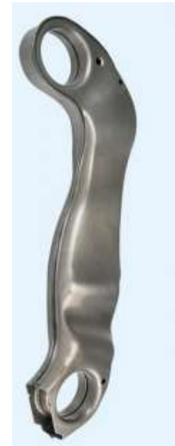
This axle component found on a Mercedes C Class sedan was laser hybrid welded at 177 IPM (4.5 m/min.) with a wire feed rate of 235 IPM (6.0 m/min.) Image source: https://www.thefabricator.com/article/laserwelding/a-look-at-laser-hybrid-welding-in-the-automotive-industry .
