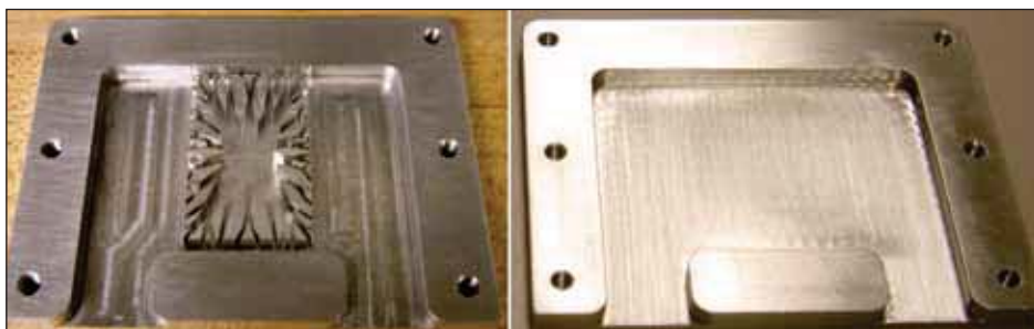
Figure 3. Prototype aluminum cold plates with (left) and without (right) the hierarchical microchannel topology.
