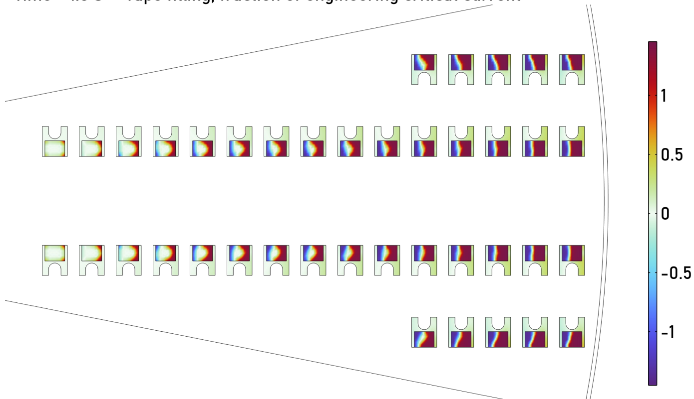
Figure 2 : Tape filling of a 2D slice of the TF centre column near the end of the CS, after 1.8s of current ramping at a temperature of 40K. The current perpendicular to the plane is plotted, normalized to the local engineering critical current.
