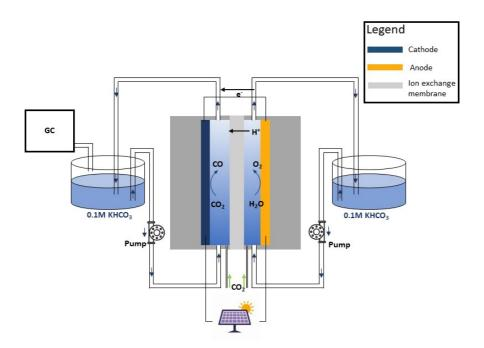
**Figure 2**: Simplified diagram of the experimental setup, with photovoltaics connected to cathode and anode as electric source.
