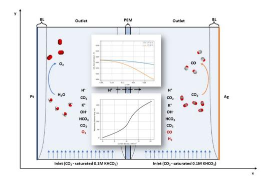
**Figure 1**: Simulation domain of the electrochemical cell, with the main chemical species and electrochemical reactions occurring at the cathode (Ag) and anode (Pt).
