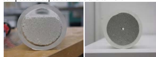
Figure 2. Cross sections of two different flow channel geometries used in tests: Segmental erosion channel (left) and hole erosion set-up (right). The diameter of the cylindrical block is 49.5 mm, and the diameter of pinhole on right hand side is 4mm.
