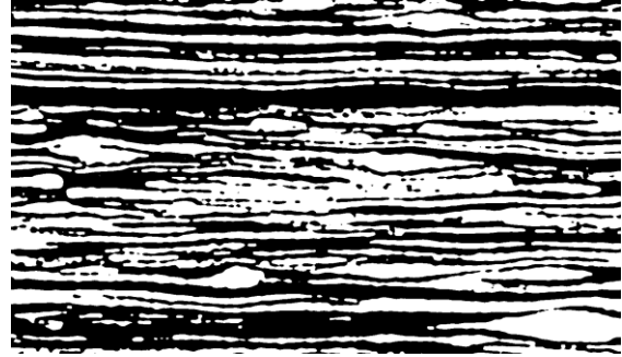
Figure 2. Microstructure of duplex stainless steel implemented in the model to define micro(x,y) .
