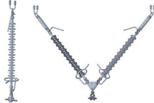
Figure 1. Suspension string and V-type suspension string with a composite insulator [1]
