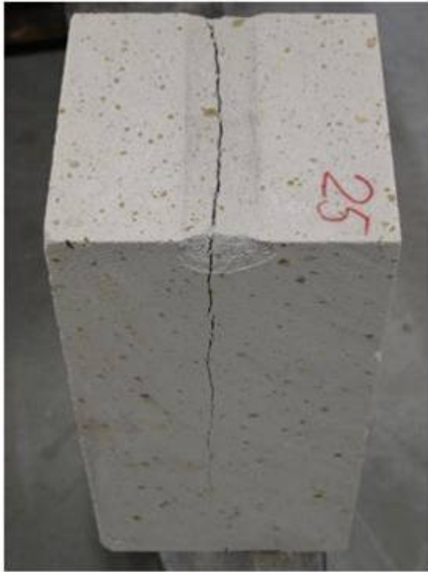
Figure 2: Split specimen with traces of centre strip after testing
