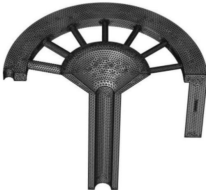
Figure 2: Flow path of the mid section and element distribution.
