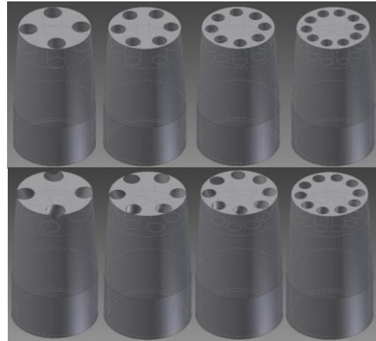
Figure 2. The applied nozzles first row - straight design, second row - swirled design
