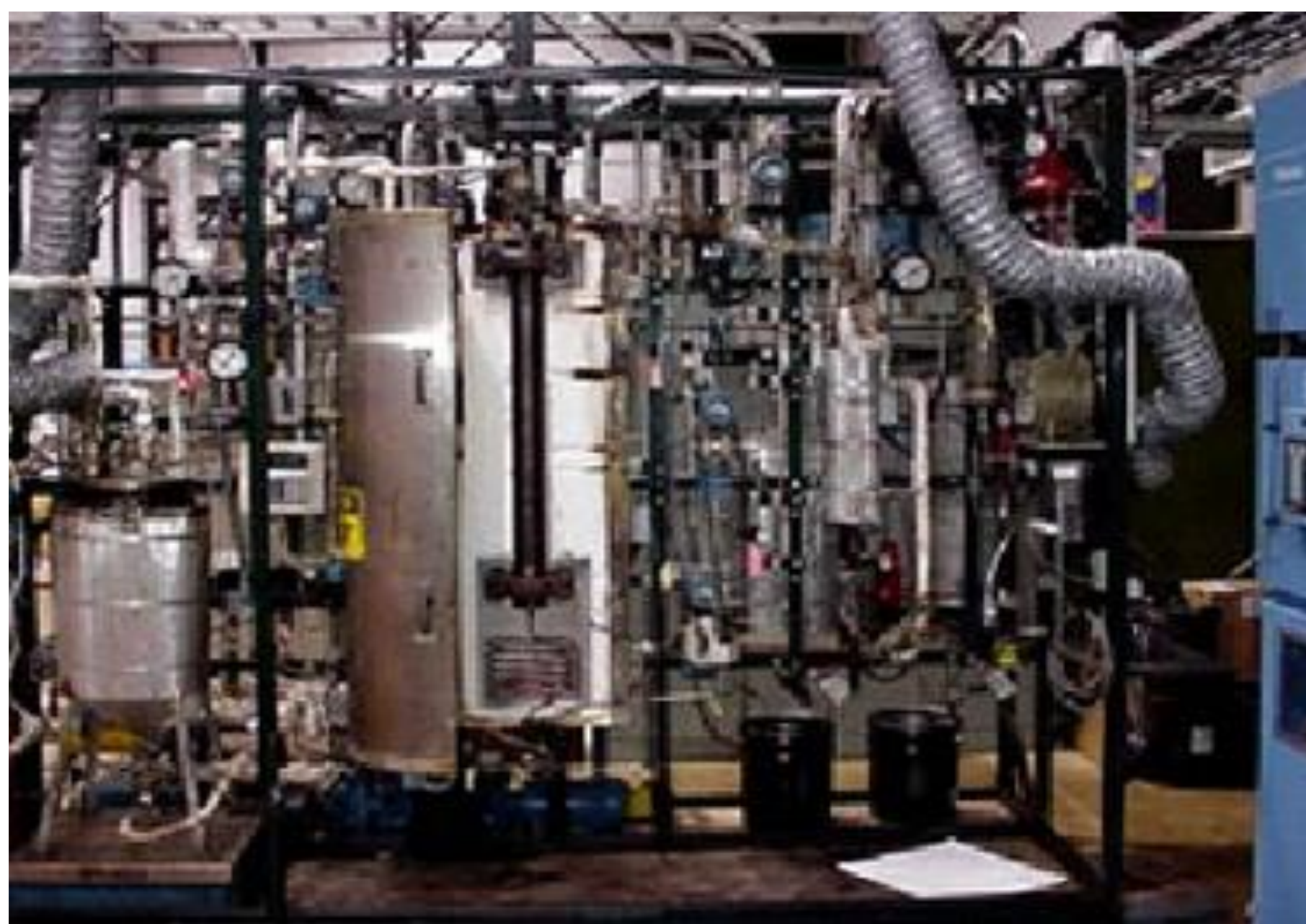
Figure 1. Pilot Unit from the University of Tulsa Delayed coking project, showing the coke drum and the furnace.
