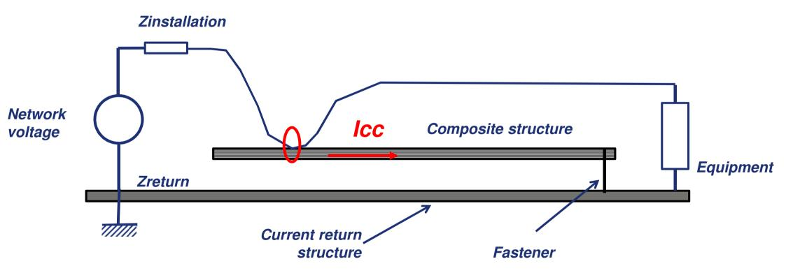
Design of a safe aircraft installation + protection devices => short-circuit has **no consequence**.
