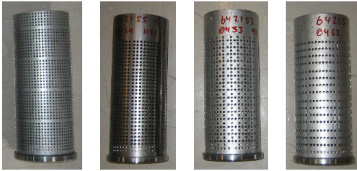
Figure 16. The perforated pipes used to verify the simulations. From left: \text{Ø}3 25.0%, \text{Ø}4 30.7%, \text{Ø}4 23.0%, \text{Ø}4 15.3%.
