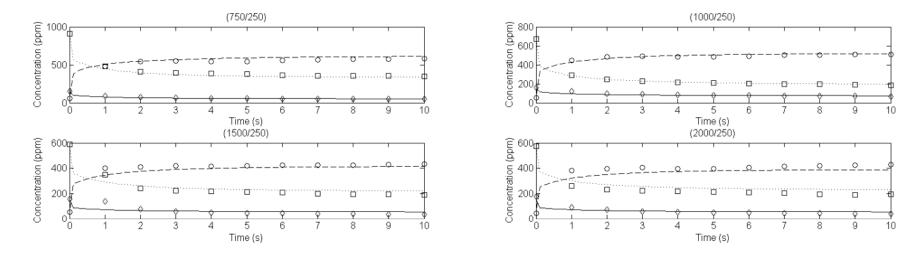
Comparison between the experimental observed and the model predicted outlet concentrations. Observed  $[NO_2]$  ( $\circ$ ); [NO] ( $\Box$ );  $[C_3H_6]$  ( $\diamond$ ). Predicted  $[NO_2]$  (---); [NO] ( $\cdots$ );  $[C_3H_6]$  (—).
