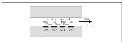
Figure 1: Cross-section of a capillary with an IDA detector utilizing redox recycling effect. The flow cell involves two working electrodes (W1 and W2), a reference electrode (RE) and a counter electrode (CE).
