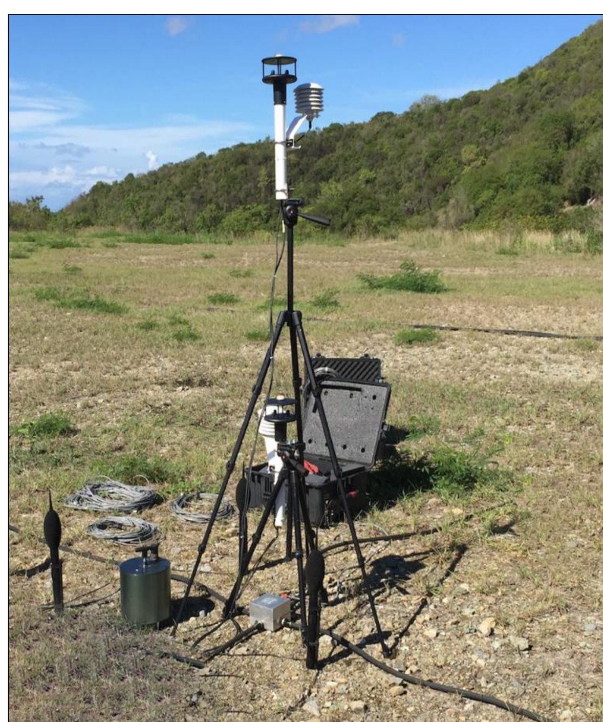
Figure 2. Seismic-Infrasound-Acoustic-Meteorological (SIAM) array
