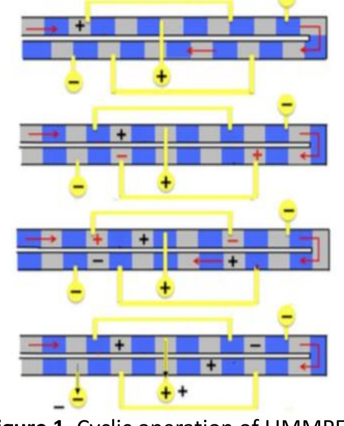
1. Droplets of oil and mercury flow in serpentine channel.
