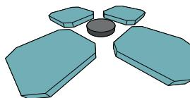
Uniform gas-liquid mixture (gas-metal or gas-alloy) in which the volume fraction of the liquid phase is small (10-20%: wet foam, <10% dry foam)
