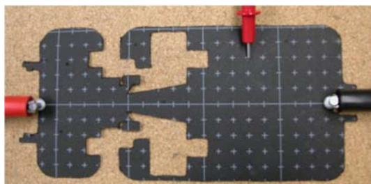
**Figure 1** Horizontal tank fixture cross-section in conductive paper.
