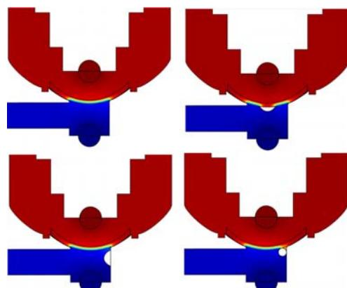
**Figure 6** Vertical fixture bubble simulations (clockwise from top left) lens mounted; bubble in center; bubble in corner and bubble along edge.
