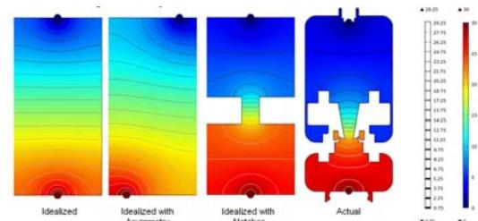
**Figure 3** Calculated 2D field maps of horizontal cross sections visualizing geometric design element affects on the electric potential field for the horizontal tank design.
