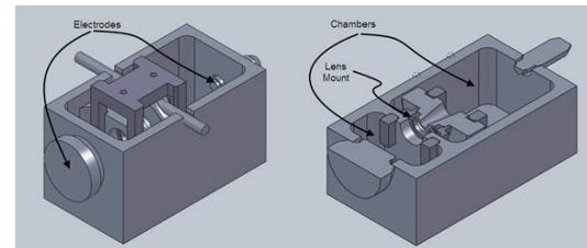
**Figure 2** Horizontal tank fixture CAD model.
