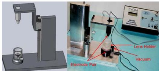
**Figure 5** Vertical Fixture CAD modal and prototype.
