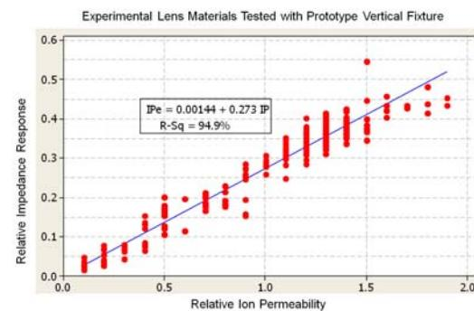
**Figure 6** Impedance response of experimental contact lens materials using the prototype vertical fixture compared to a traditional method of characterizing ion permeability.
