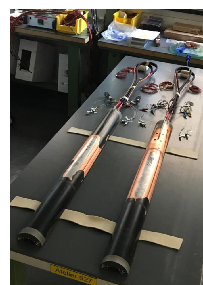
Feather-M2 coils (Courtesy of J. Van Nugteren)
